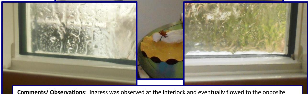
**Comments/ Observations:** Ingress was observed at the interlock and eventually flowed to the opposite corner. Failure did not occur however as the water evacuated during the rest periods in between test cycles. Specimen 3 was awarded a technical pass.
