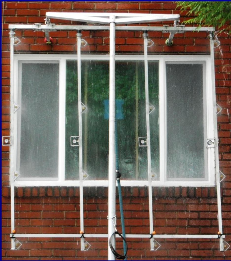
Specimen 3 is a VPI window that measures 50" X 32". It has an AAMA performance grade rating of LC 30.
